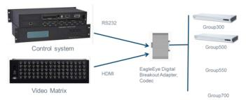
The two EagleEye Digital Breakout Adapters can be used together to extend the distance from EagleEye IV cameras to the Group Series codecs.
